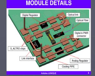
Realistic design of pad PCB with all components 64ch S-ALTROs replaced by proper FPGAs and OP amp/ADC as current load and heat source. Connect pads to the FPGA analog outputs Try cooling by the 2-phase CO2 cooling (AMS and LHCB: Bart Verlaat/Nikhef) Test also digital software model/communication in FPGA Test in high magnetic field
