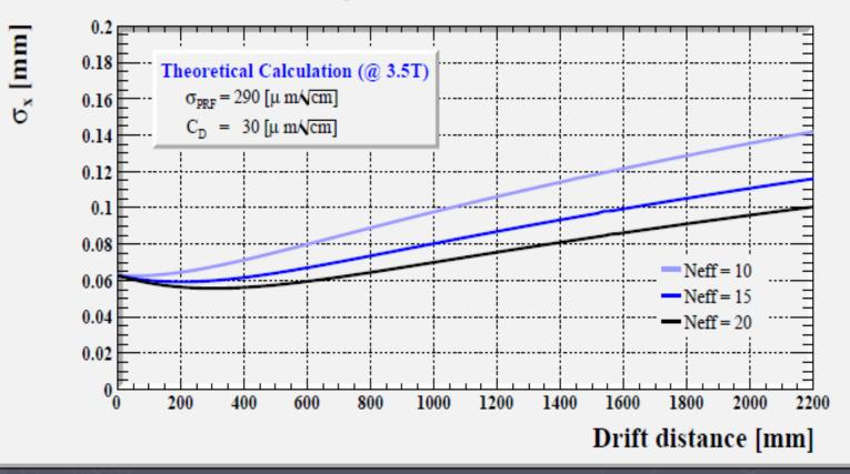
These calculations are for GEM with 6mm long pads. The dependence on Neff is similar for MicroMEGAS in large drift distance. Neff, The effcetive number of primary electrons contribute to position resolution, measured both for MicroMEGAS and GEM are around 20 (@1T).
