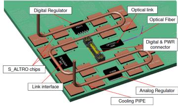
Option of Cooling: 2-phase CO2 cooling/traditional H2O cooling
