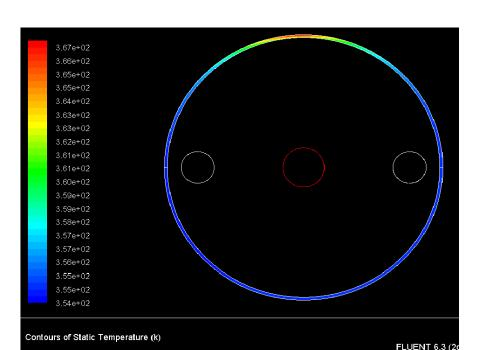
Temperature distribution in the vessel at z = 4.2m for the 0.45m radial beam location
