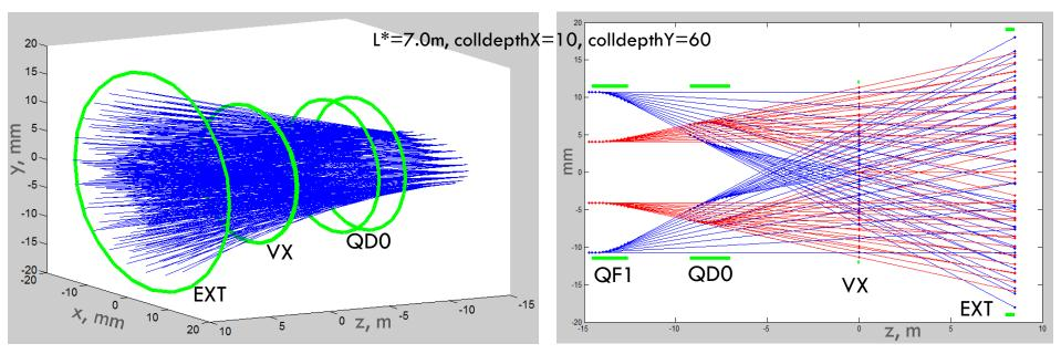
Rays show trajectories of possible SR photons. Amount of rays is not quantitative.
