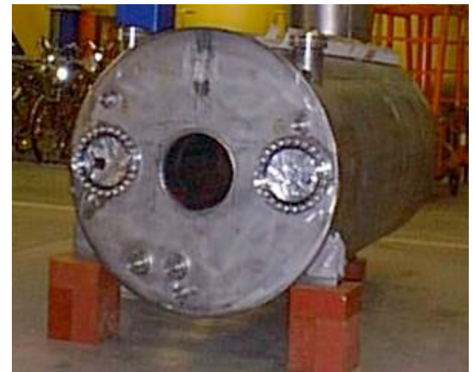
5T Magnet with 28cm inner diameter
