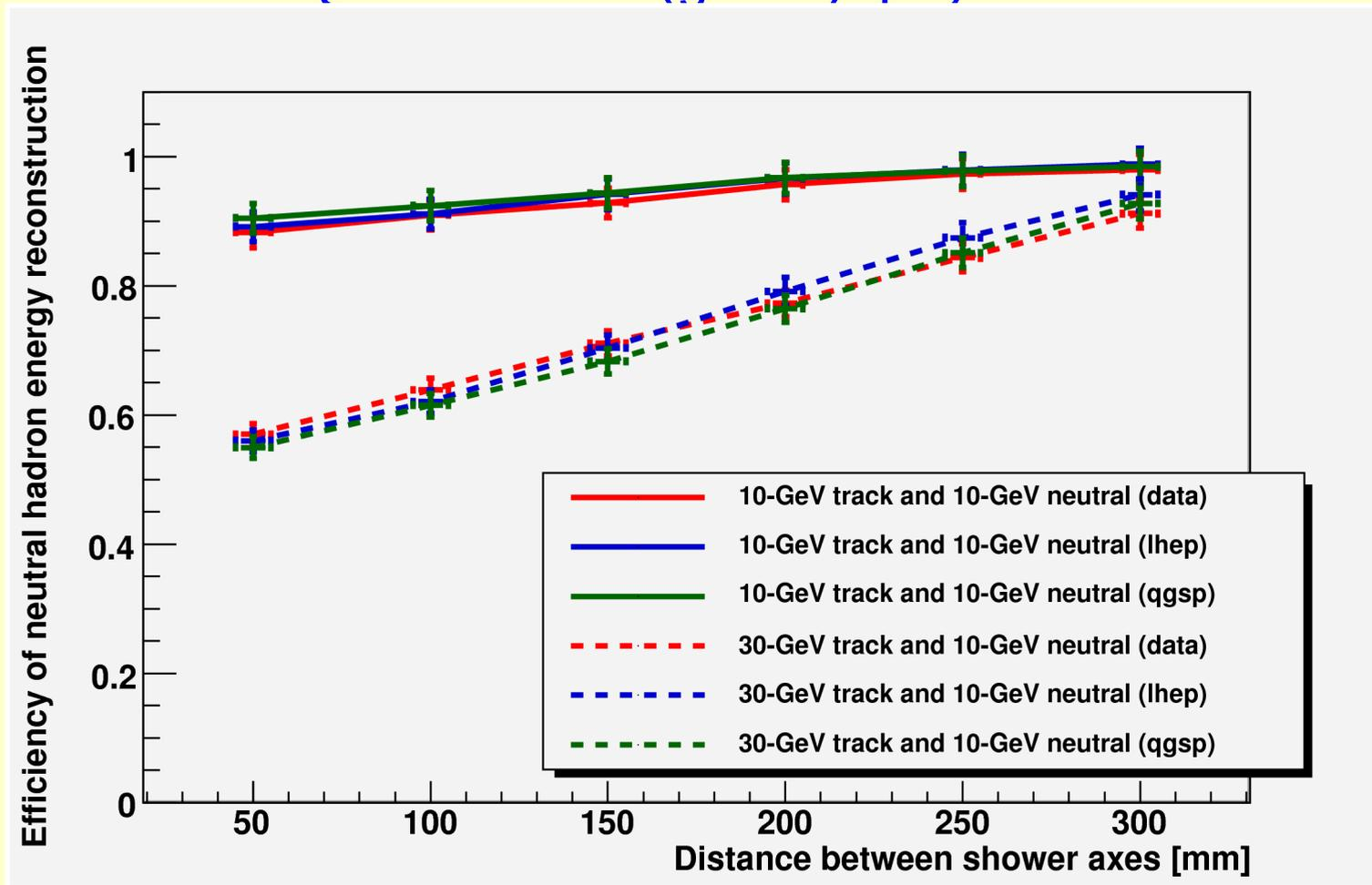
RMS<sub>90</sub> deviation for *recovered energy* of neutral hadron from its *measured energy* (left) and the efficiency of the neutral hadron energy reconstruction within 3 standard deviation (right) vs the neutral hadron energy in the vicinity of the 10 GeV charged hadron (red lines) and the 30 GeV charged hadron (blue lines) for typical distances between neutral and charged hadrons
