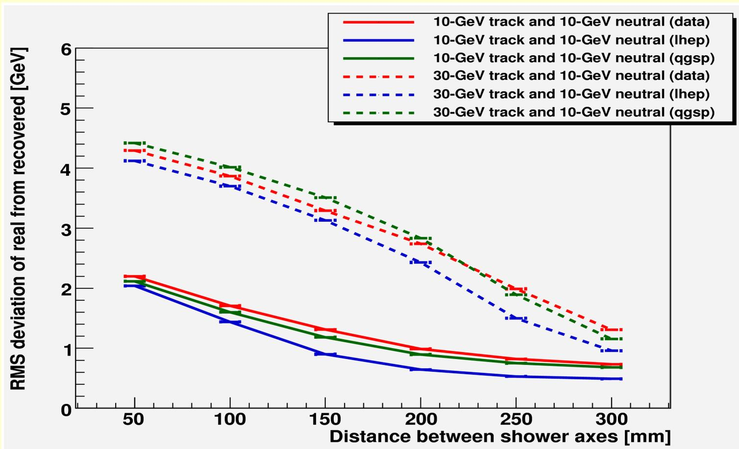
Efficiency of the neutral 10 GeV hadron energy reconstruction within 3 standard deviations vs. the distance from the charged 10 GeV (continuous line) and the 30 GeV (dashed line) hadron for beam data (red) and for Monte Carlo simulated data, for both LHEP (blue) and QGSP-BERT (green) physics lists
