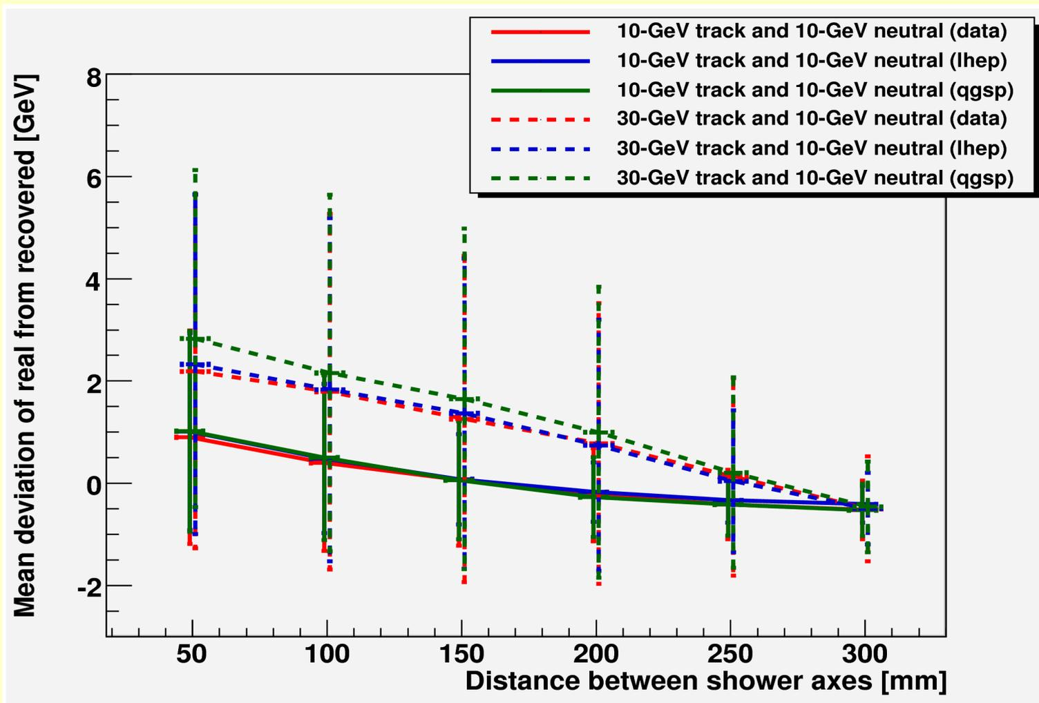
RMS<sub>90</sub> deviation for the *recovered energy* of the neutral 10 GeV hadron from its *measured energy* vs. the distance from the charged 10 GeV (continuous line) and the 30 GeV (dashed line) hadron for beam data (red) and for Monte Carlo simulated data, for both LHEP (blue) and QGSP-BERT (green) physics lists
