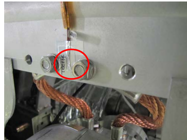
Connection of 5K thermal anchors to 5 K shield. Indium sheet was sandwiched. T-sensor is Cernox.
