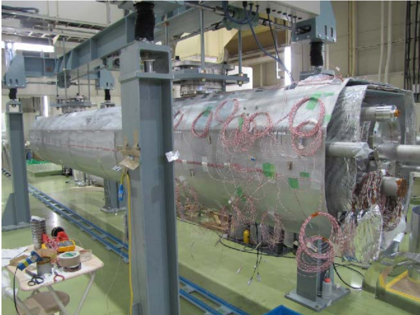
Thermal sensors on the 80K shield (Cu-Constantan thermo-couples)
