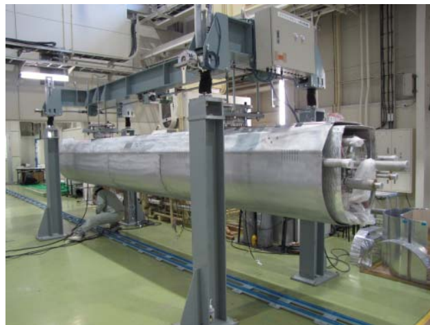
Assembling 80 K shield
