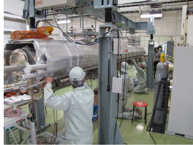
Assembling cool-down/warm-up pipe
