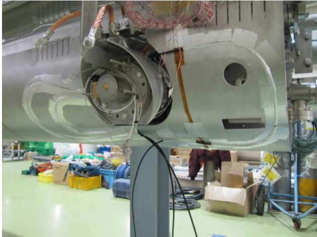
Thermal anchoring RF cables on the 5K shield
