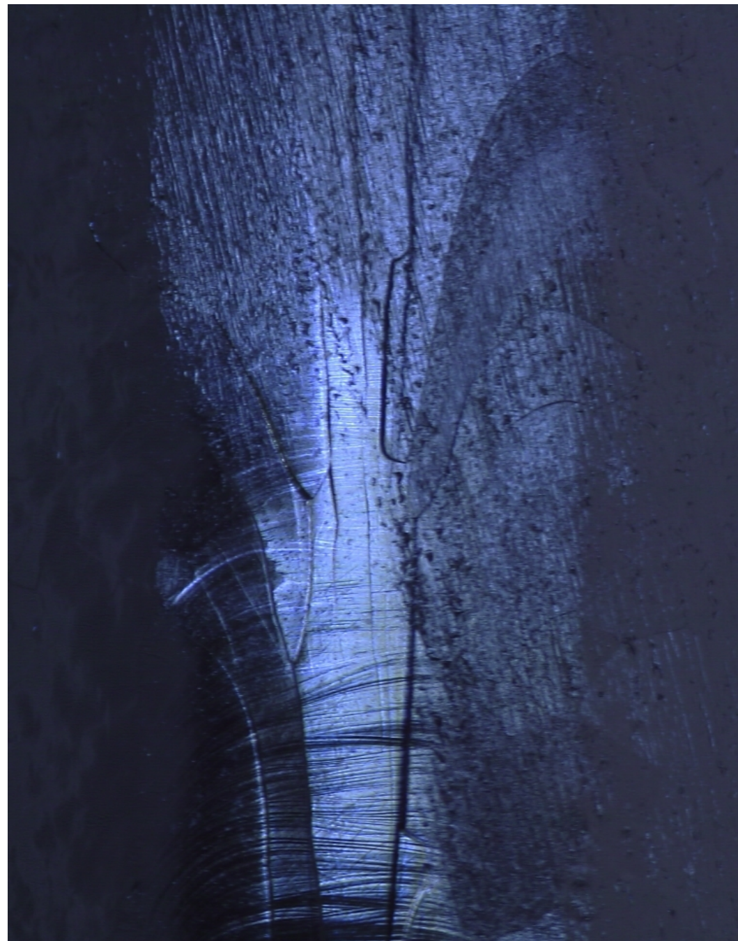
Pristine (left) and partially machined (right) iris weld
