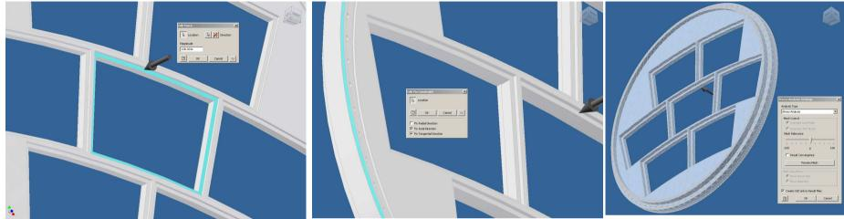
(left) The applied force was 100N (22 lbs) "evenly" distributed over the indicated face on the endplate. This applied force can be easily reproduced on the prototype.
