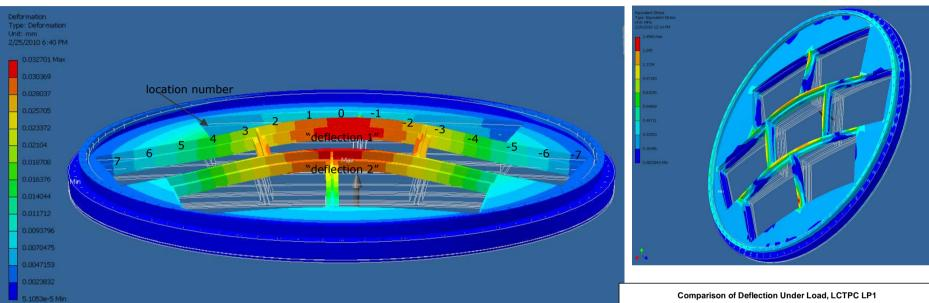
(left) **Measured** values of the deflection of the LP1 endplate are compared to the FEA results:
