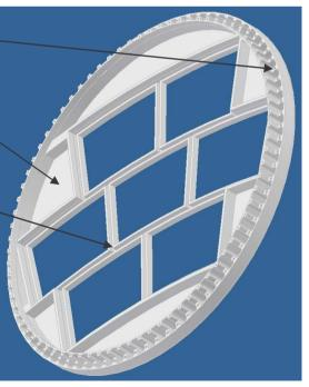
A new, functional, LCTPC LP1 endplate is being designed with this model.
