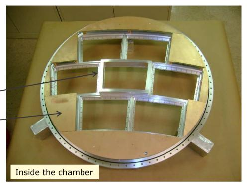
The endplate construction was developed to provide the precision required for the ILD; precision features are **accurate to ~30 microns**,
