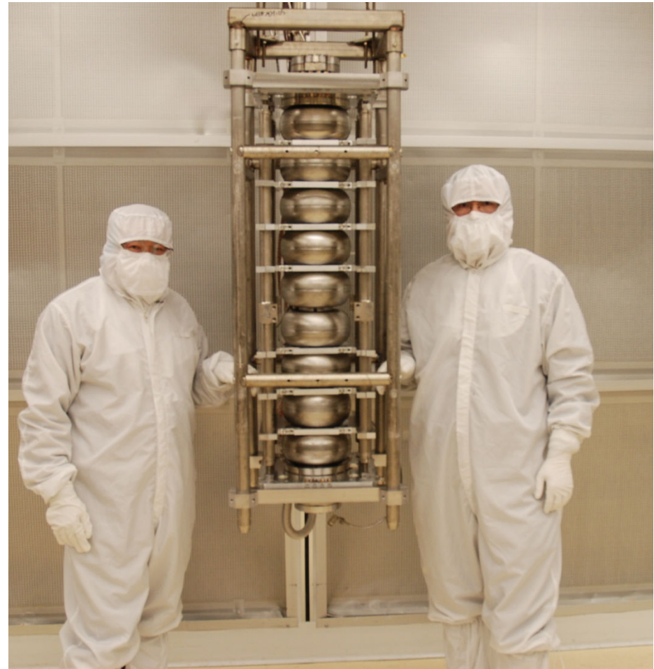
KEK Ichiro7 cavity finished clean room assembly at JLab
