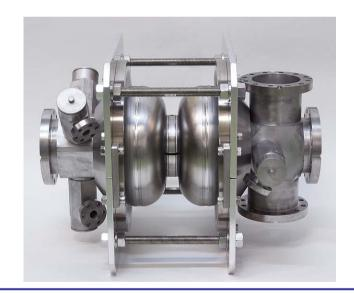
Two step test for both cavities: (1) Without HOM pickup probe, (2) With HOM pickup probe.
