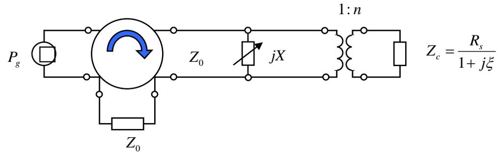
Figure 1: *Equivalent circuit of cavity powered through a circulator with the variable obstacle (no moving along waveguide)*
