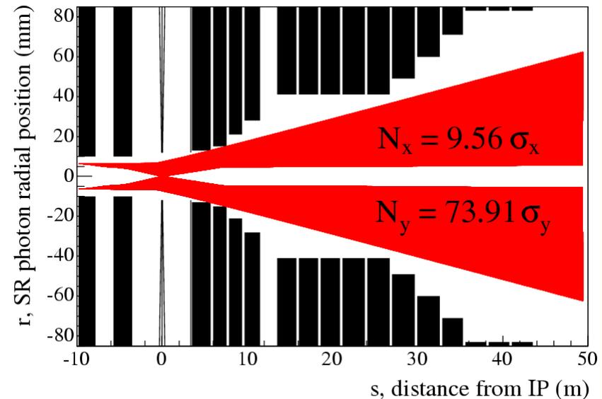
**Example of SR rays from beam halo in IR apertures**
