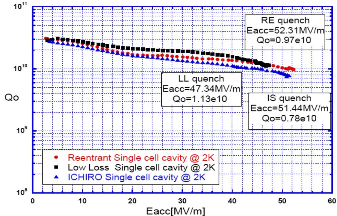
Figure 3: The results of high gradient measurements.
