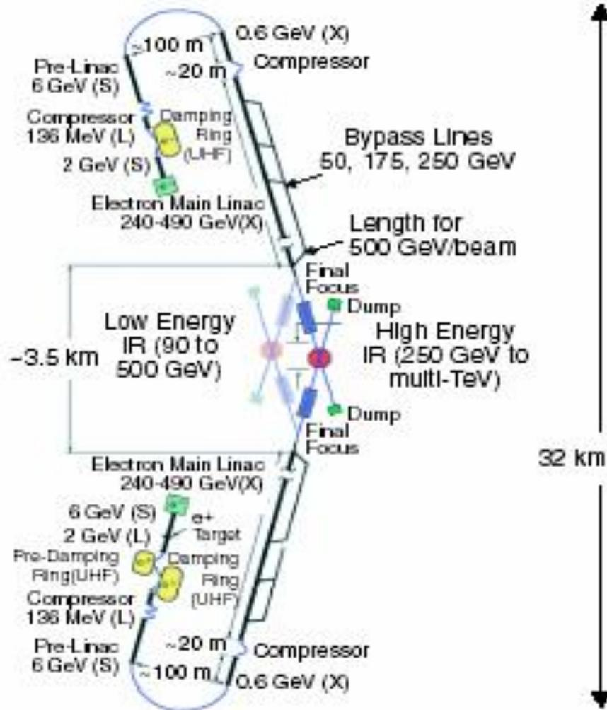
The JLC-X and NLC essentially a unified single design with common parameters
