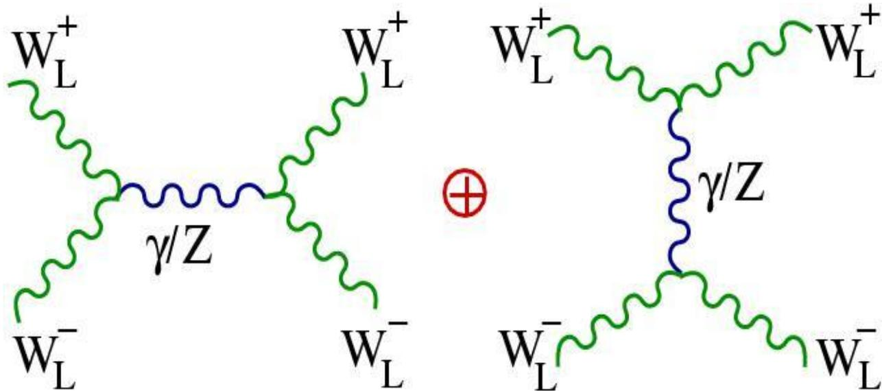
**Cross section for WW scattering violates unitarity at  $\sim 1.2$  TeV, unless there are new resonances**
