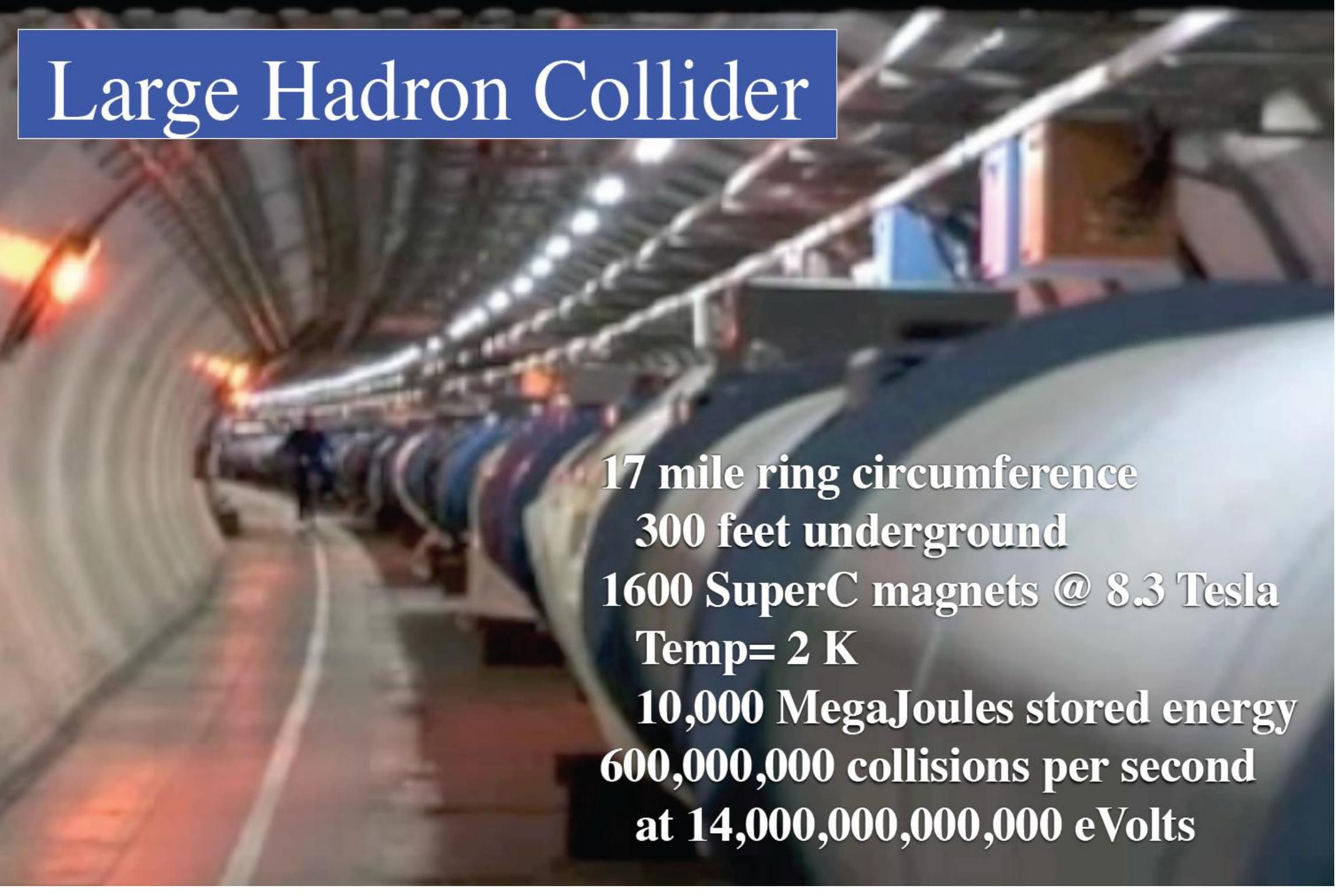
The image shows the interior of the Large Hadron Collider tunnel. The tunnel is a long, curved passage with a series of large, cylindrical superconducting magnets lining the walls. The magnets are arranged in a circular pattern, and the tunnel is illuminated by warm, orange lights. The perspective is from the end of the tunnel, looking down its length.
