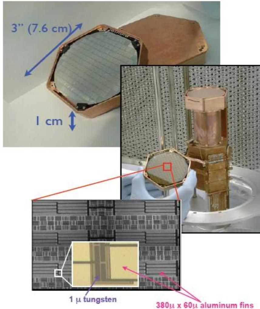
The CDMS experiments measures the recoil energy imparted to detector nuclei through WIMP-nucleon collisions by employing sensitive phonon detection equipment coupled to arrays of cryogenic germanium and silicon crystals.
