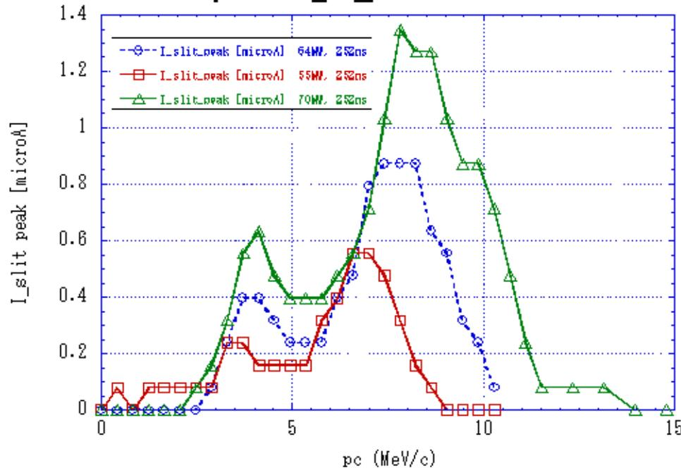
Measured dark current energy spectrum at downstream
