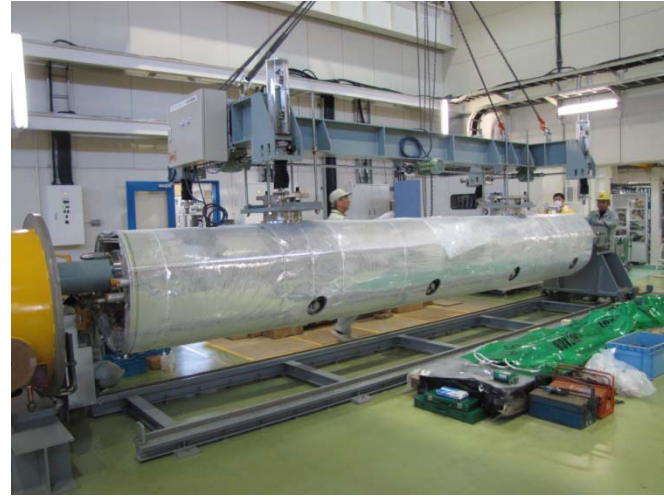
Moving the cold mass to the insertion area
