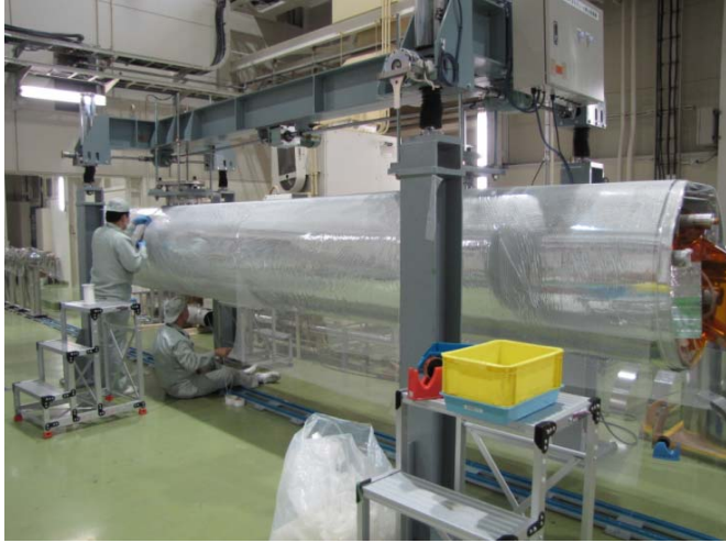
Wrapping the SI around the 80K shield
