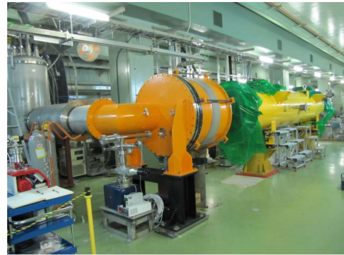
Setting the Module-C on the support stand in the STF tunnel.
