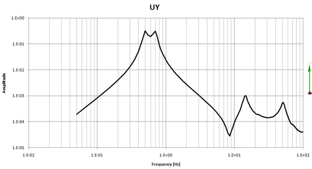
There is a good decoupling between horizontal & vertical directions
