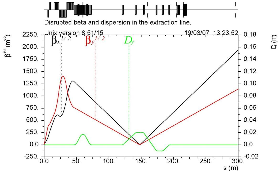
Optical  $\beta$  functions and vertical momentum dispersion  $D_y$  in the 14 mrad extraction line from IP to the dump, shown for the 250 GeV nominal disrupted beam.
