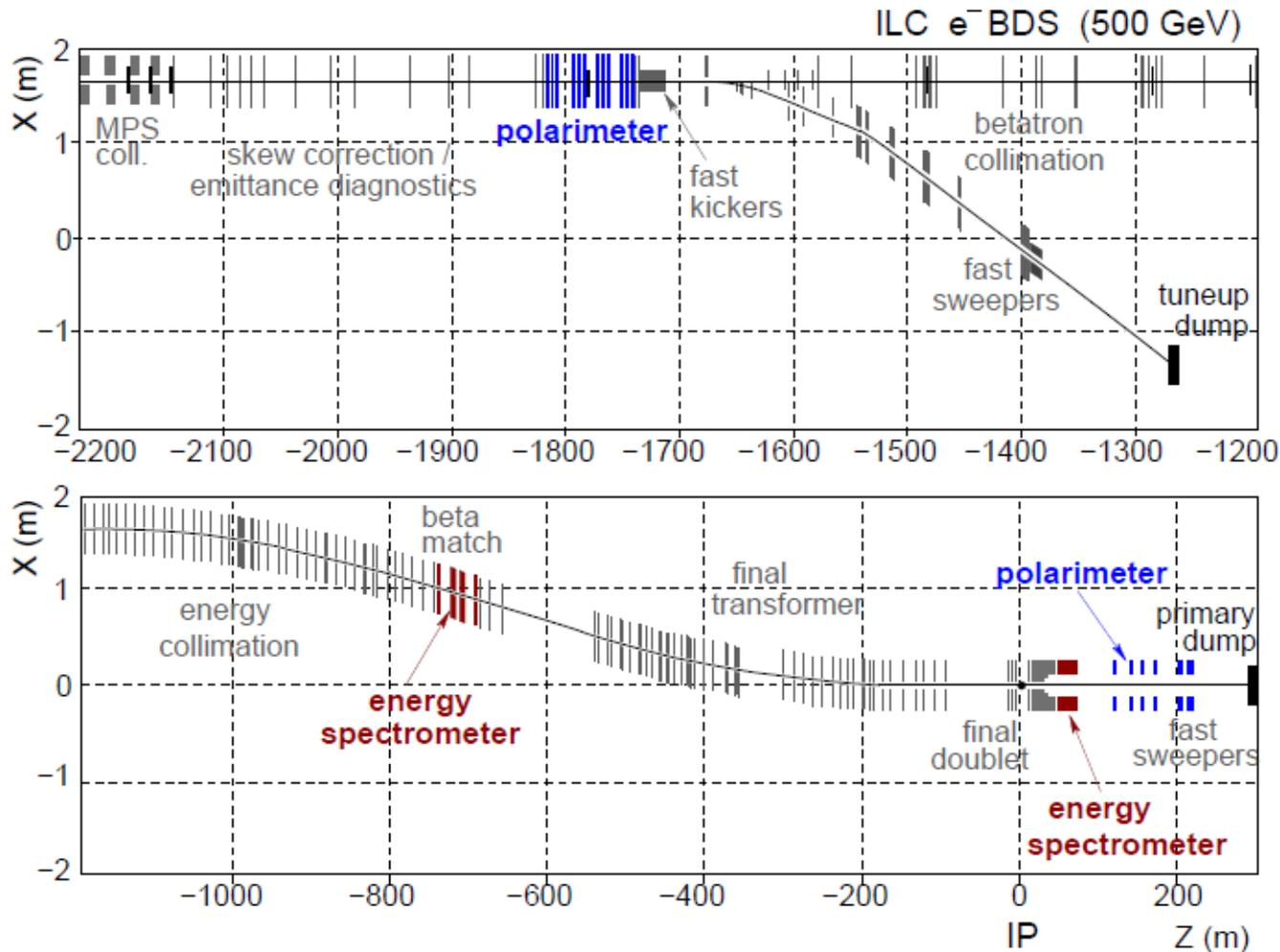
Beam Delivery System (BDS) as described in the RDR. The upper part shows the region from 2200 m to 1200 m upstream of the  $e^+e^-$  IP, including the polarimeter chicane at 1800 m. The lower part shows the region from 1200 m upstream to 400 m downstream of the IP, including the upstream energy spectrometer at 700 m as well as the extraction line energy spectrometer and polarimeter around 100 m downstream of the IP located at  $z = 0$  m.
