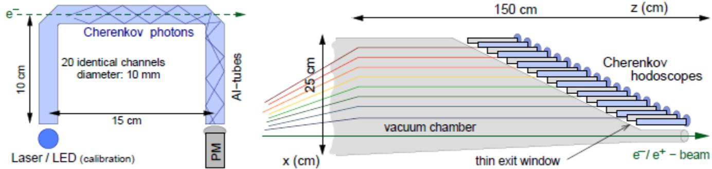
*Schematic of a single gas tube (left) and the complete hodoscope array covering the tapered exit window (right) as foreseen for the Cherenkov detectors of both polarimeters.*
