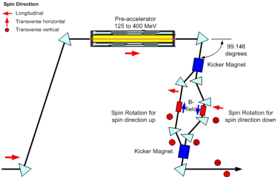
After a bend of **99.146 degrees** a copper wound solenoid of **2.096 Tesla meters 2.2 meters** long with an axial field of **9.53 Kilogauss** will rotate the spin from the transverse horizontal direction to the vertical. Criteria for the kicker magnets for spin flip and tunnel space is much less demanding at **400 MeV** than at **5 GeV**.
