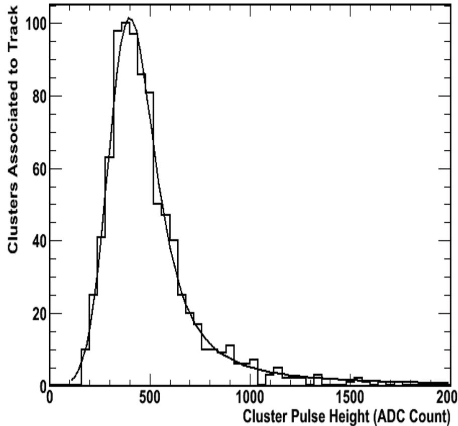
Cluster reconstruction using double S/N threshold (seed and neighbouring pixels) (seed S/N > 10 and  $N_{\text{pixels}} > 1$ )
