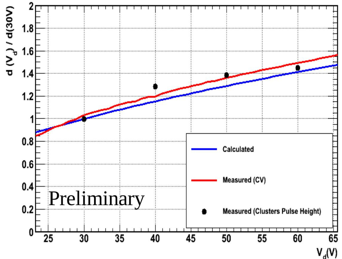
Calculated depletion from nominal resistivity (200  $\Omega$  cm);
