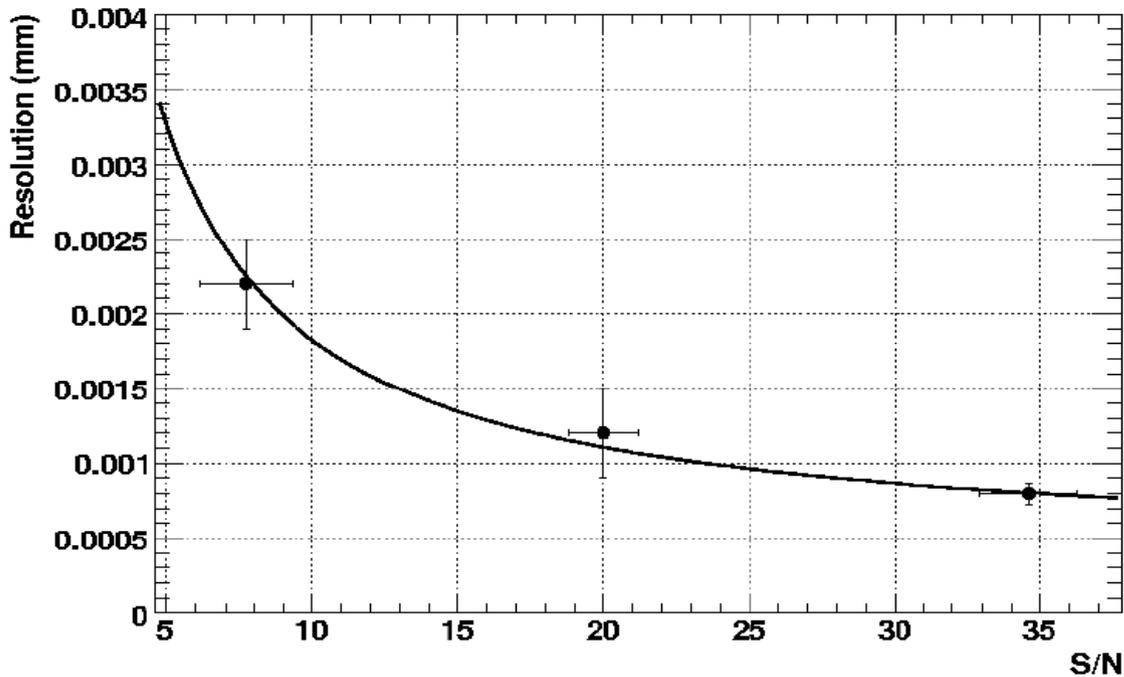
First estimate single point resolution by performing pixel scans on SOImager chip with 1060 nm laser focused to  $\sim 5 \mu\text{m}$  spot at various intensities to simulate m.i.p. charge deposition;
