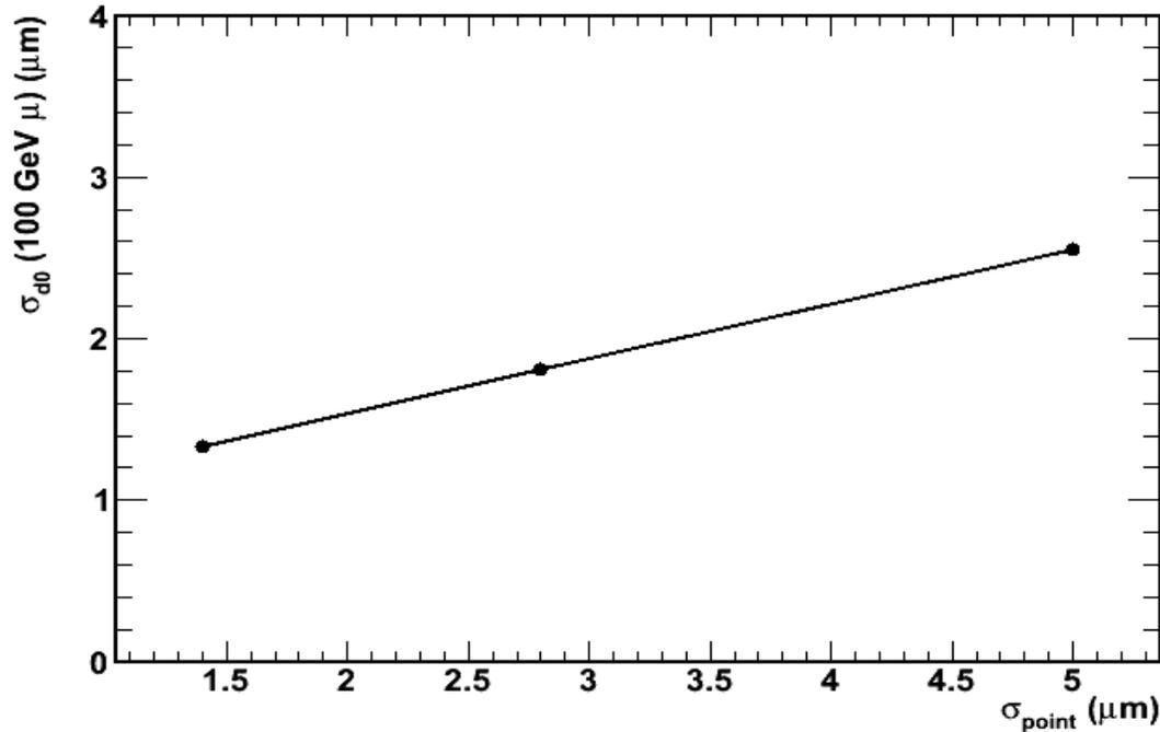
Scaling of asymptotic R- $\Phi$  impact parameter resolution (a) with single point resolution for a three double-layered barrel VXD in the CLIC geometry (100 GeV single muons with Mokka+MarlinReco);
