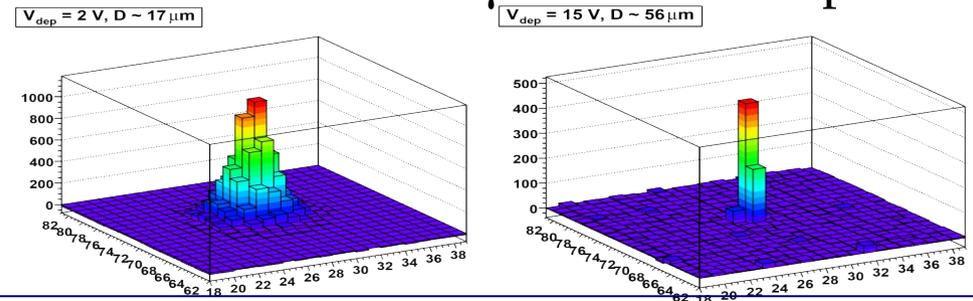
Results of first pixel detector test structures in OKI SOI technology encouraging but two main issues emerged: transistor back-gating and charge trapped in thick BOX
