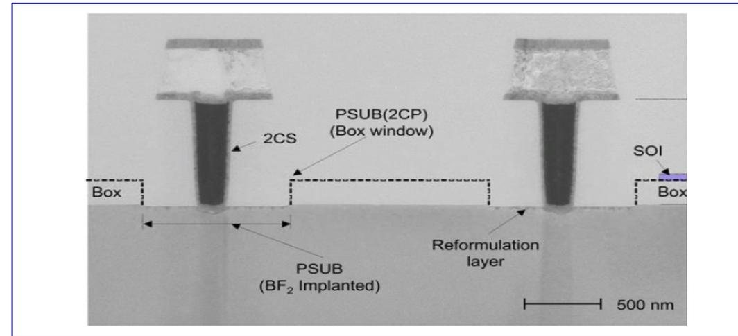
Thick fully depleted substrate gives large collected charge, faster collection time and small charge spread compared to conventional CMOS APS on low-res epi:
