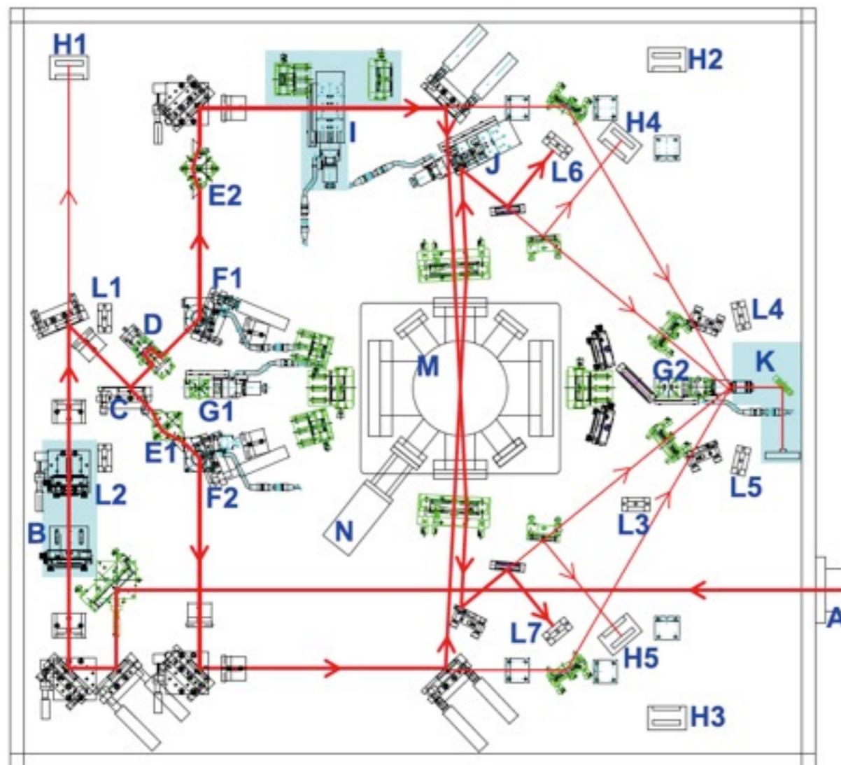
Laser path diagram (174 deg crossing angle)
