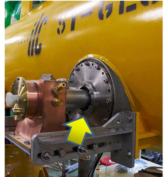
The connection flange design is dependent on the input coupler design. For accommodating both types of input coupler, the additional intermediate flange is necessary.
