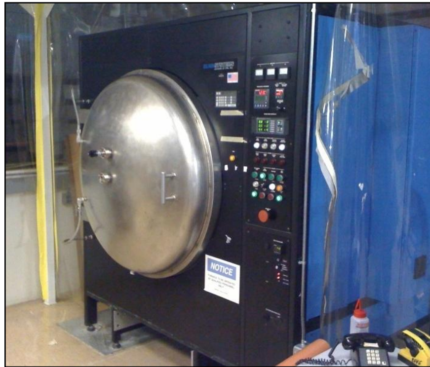
Jlab oven currently used for hydrogen degassing of all Americas Region cavities
