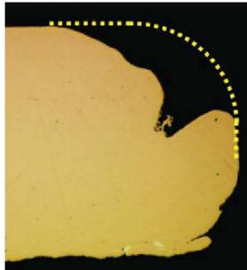
Field electron emission plays a significant role in the arcing phenomenon[1]. Resistive heating, due to the emission current, can cause melting to occur, providing evaporated atoms to build up plasma. If a microscopic protrusion is present on the surface, the threshold of the applied electric field for plasma formation is lower because of the local enhancement of the electric field above the tip.
