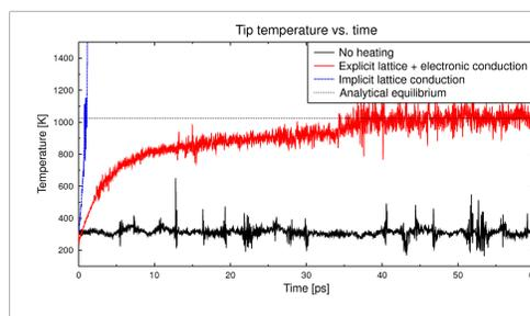
Simulations show that electronic heat conduction must be considered explicitly to obtain analytically predicted temperatures.
