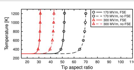
Maximum temperature is a function of tip aspect ratio:
