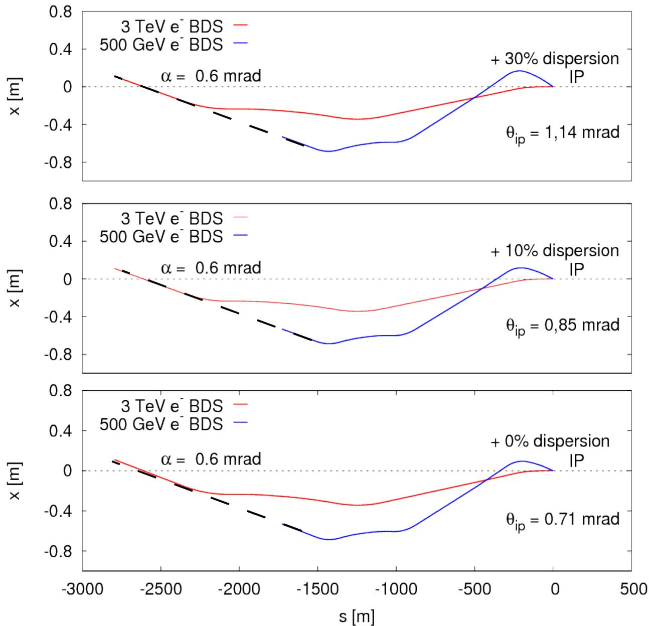
To maintain the Diagnostics section aligned with the LINAC the rotation angle around the IP increases as the dispersion is increased.
