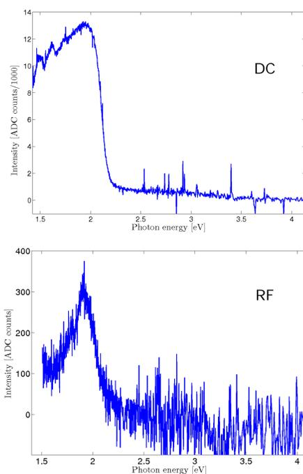
OTR spectrum in dc and rf. Shoulder at 2.1eV created by Cu interband transition.
