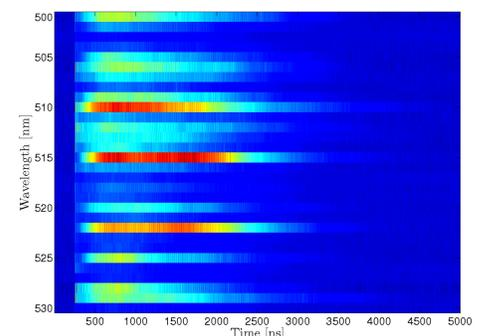
Time resolved wavelength interval of a dc breakdown on a Cu sample.
