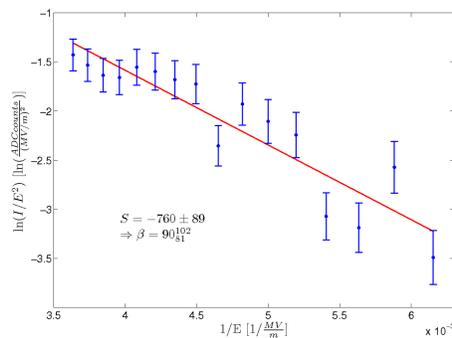
Example of a  $\beta$ -fit using OTR light intensities.
