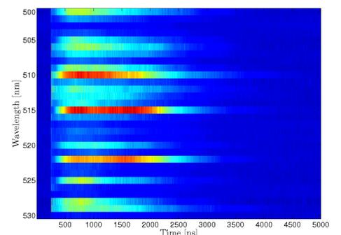
Time resolved wavelength interval of a dc breakdown on a Cu sample.
