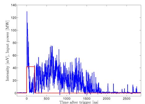
Total emitted light intensity (blue) and rf input power (red) of an rf breakdown, the first sharp peak can be attributed to strong OTR.
