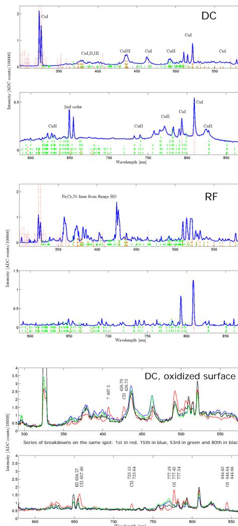
Breakdown spectrum in dc and rf on Cu. Removal of CuO layer (~150nm) due to conditioning.
