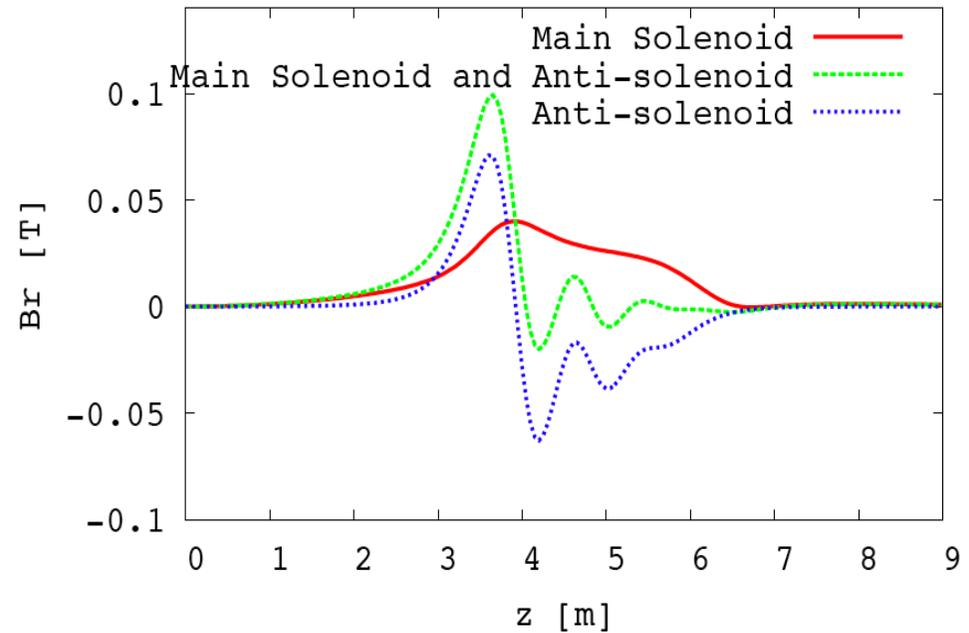
It surrounds QD0 and is made of several coils, powered with different currents. It also compensates to a large extent the effect of the main solenoid on the beams.
