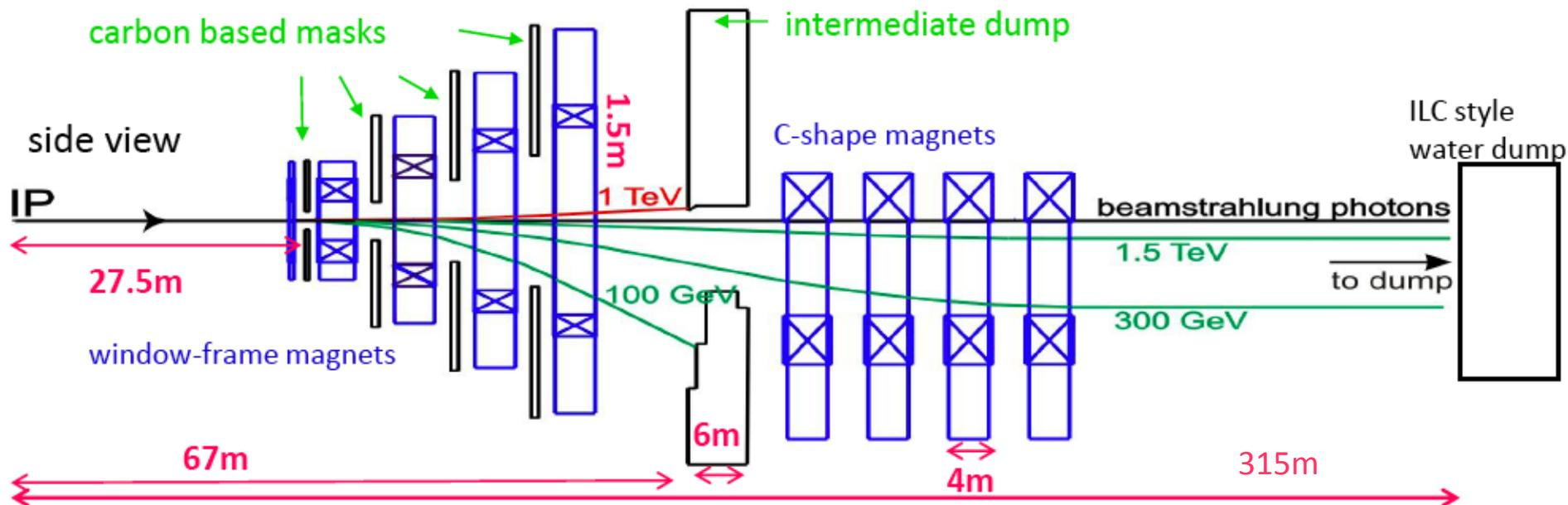
1. Separation of disrupted beam, beamstrahlung photons and particles with opposite sign from coherent pairs and particles from  $e^+e^-$  pairs with the wrong-sign charge particles
