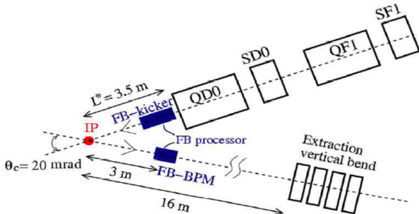
If FONT elements 3 m apart from IP, then beam time-of-flight = 10 ns
