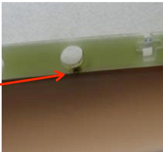
At the initial HV test washer might be at the opposite position of pad plane.
