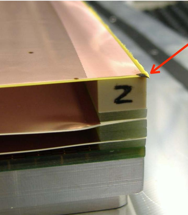
When HV trip, discharge may happen because Gate electrode is too close to Dummy surface over placed insulator help discharge
