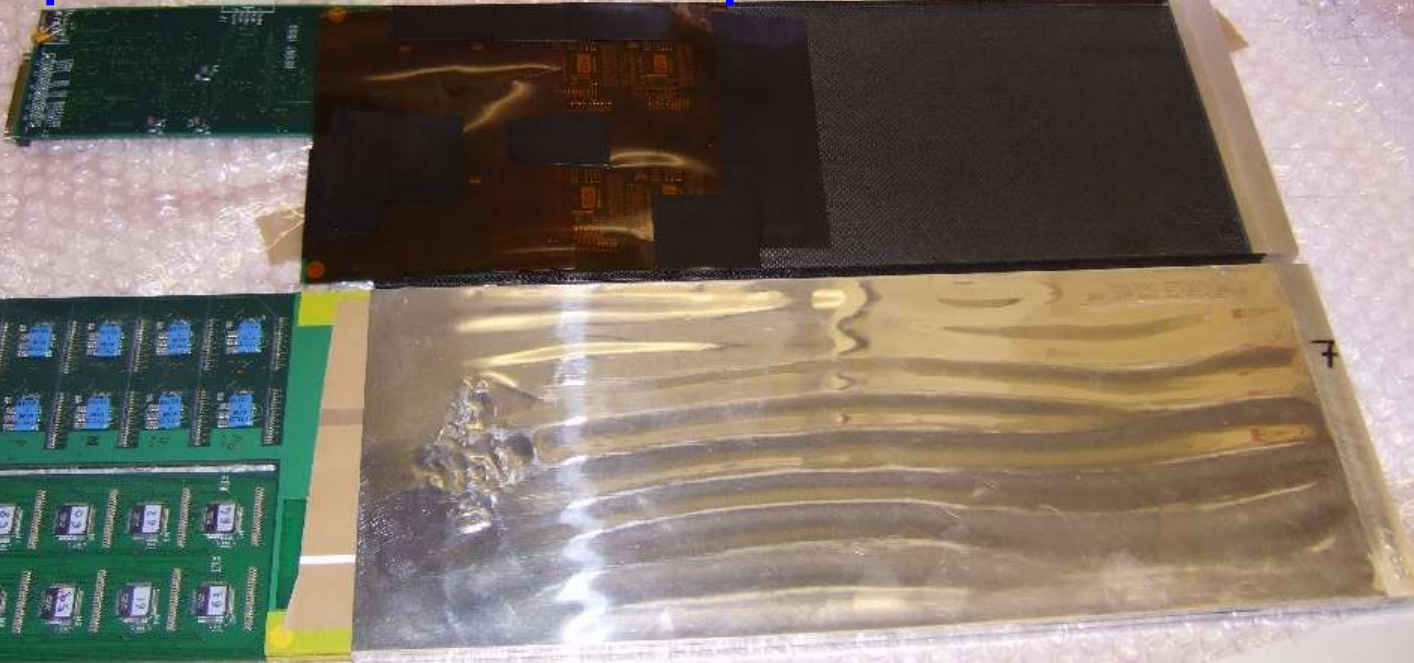
Prepared Slab - W dummy - capton and paper for electrical shielding
