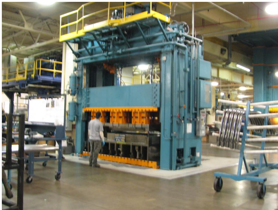
Production 4000 ton hydroforming press.
