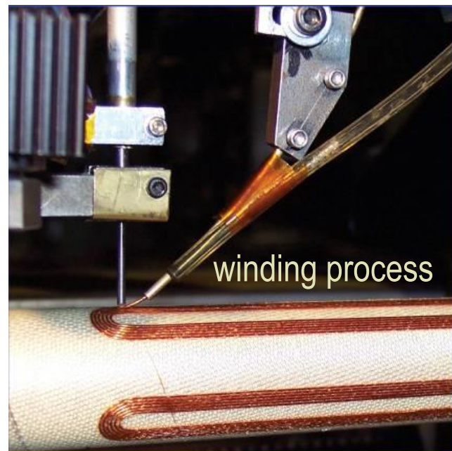
cancellation of the external field with a shield coil has been successfully demonstrated at BNL
