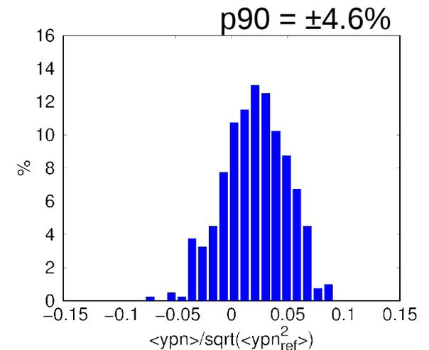
5% rms incoming electron beam jitter (Gaussian)  $\approx$  90% of cases within  $\pm 8\%$  jitter, no correction, no misalignment, plots show final distribution in normalized phase space, with ISR and short range wakes
