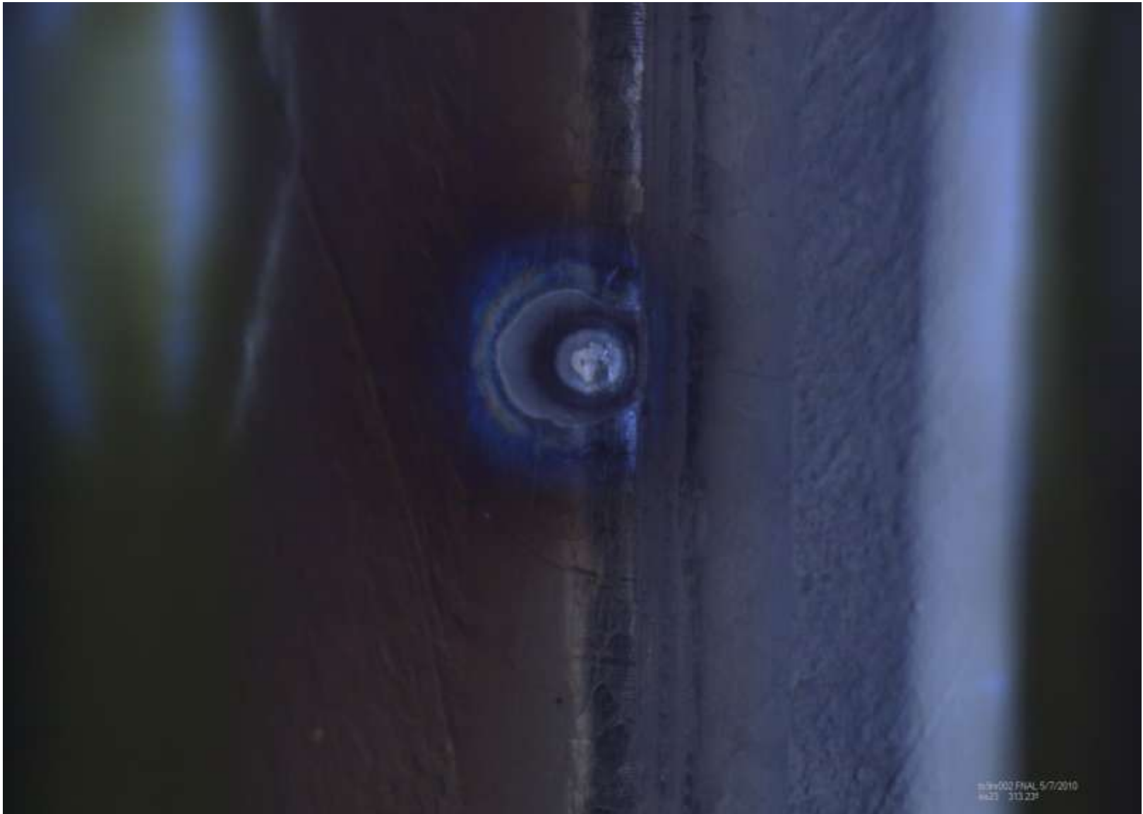
NR002: unique defect on Iris between cells 2 and 3 – BAD, this should be caught at the dumb-bell stage and the part discarded.
