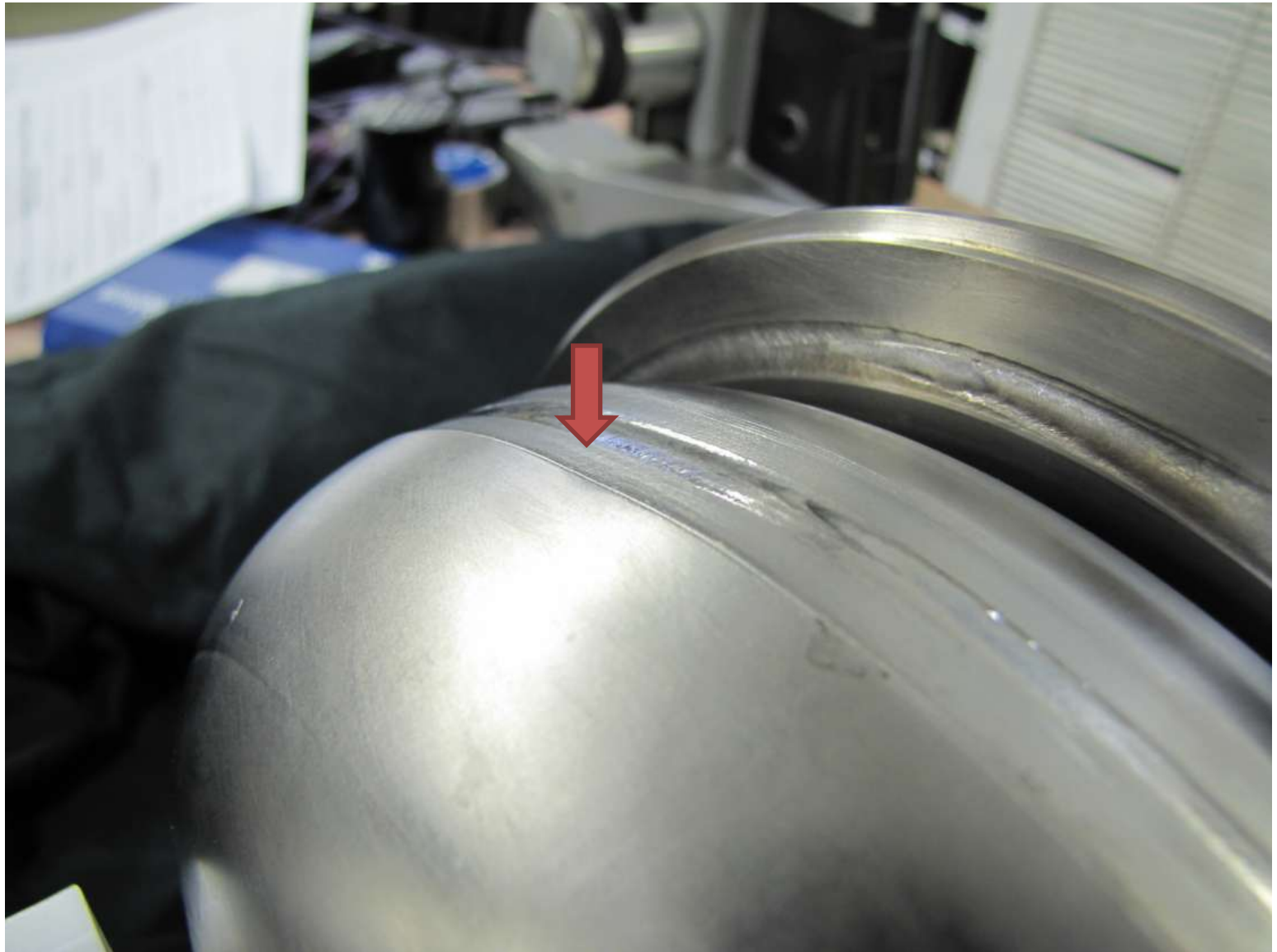
NR001: dent on end cell - BAD
