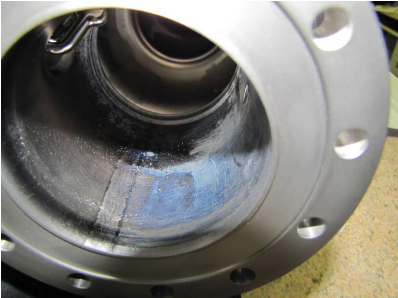
NR002: Discoloration, dirt (?) and fingerprint(?) inside beam tube at probe end - BAD .
