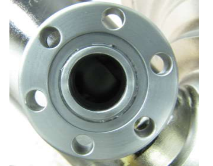
NR001 & NR002: all flanges have weld gaps and show a lot of polishing - BAD
