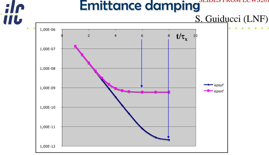
8 damping times are needed for the vertical emittance
