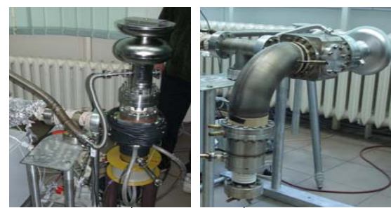
Location of the heater with lead stub for plasma formation
