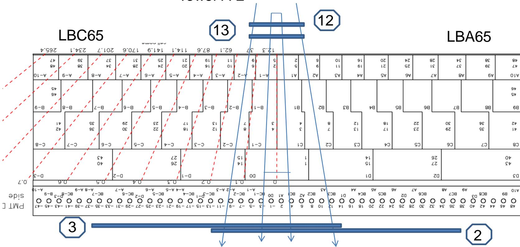
**Cosmic muons trigger: ( 12 AND 13 ) AND ( 2 OR 3 ) ( ~0.13 Hz)**
