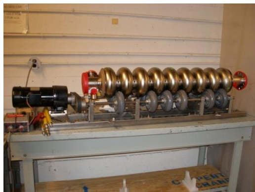
Strengthened machine. Approximate removal rate when one cell is tumbled is 15 \mu\text{m} per day.
