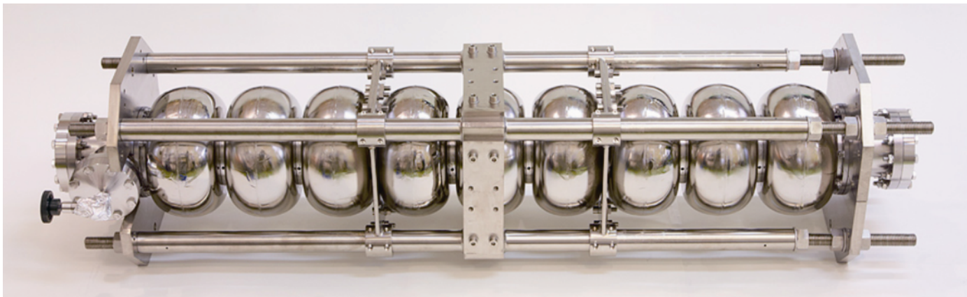
IHEP 9cell Low Loss Cavity (without HOM Couplers) IHEP_01 1st. Vertical Test 06/30-07/01/2010 Surface Treatment at IHEP Liquinox 2% (43C,3hrs), H.P.R.(8.5hrs) at KEK
