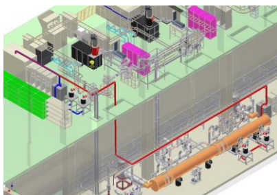
Figure 6: Layout of DRFS on S1 global. DC power supply is set upstairs and thru the HV cable, HV are applied to DRFS klystrons in the tunnel.
