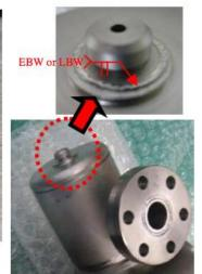
Deep drawing of HOM cup, Laser beam welding, more smooth EBW seam
