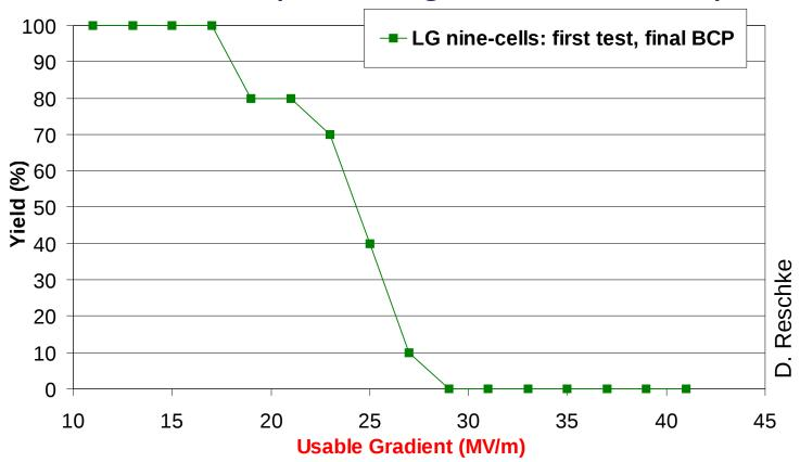
Usable gradient limited by either radiation level (1E-2 mGy/min) or 100 W input power
