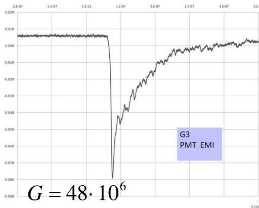
Example of signals from the two PMTs of glass #3 due to cosmics.
