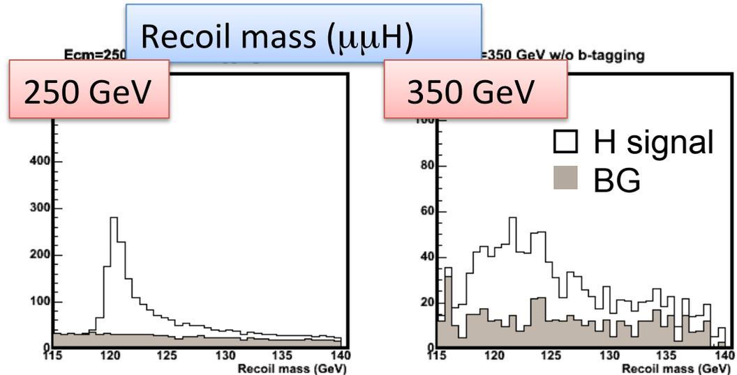
Narrow recoil mass distribution in  $\mu\mu$ H mode from better momentum resolution at  $E_{cm}=250$  GeV
