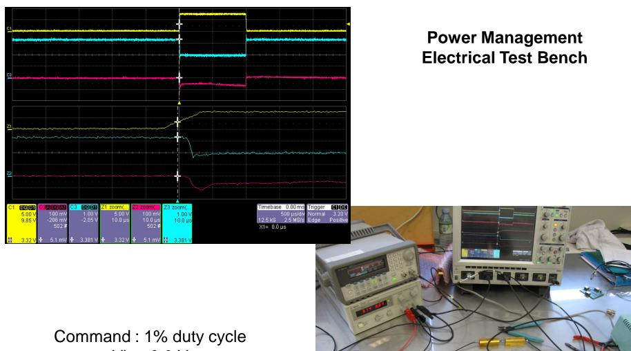
Vin= 3.3 V Load : 1 A on 1 Ohm, 1 ms, rise=1 us Vin undershoot : 100 mV
