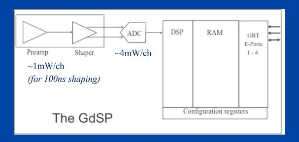
64 channels = Analog power ~ 320mW + Digital power ~ a few hundred mW. Approx. ~500mW / chip.
