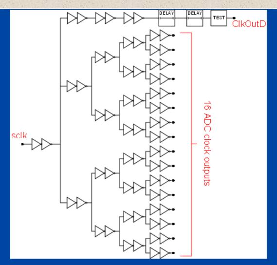
Buffer the clock to the 16 channels, deliver a delayed clock (typical: 600ps) to the digital block. Fully symmetrical structure (also in layout).
