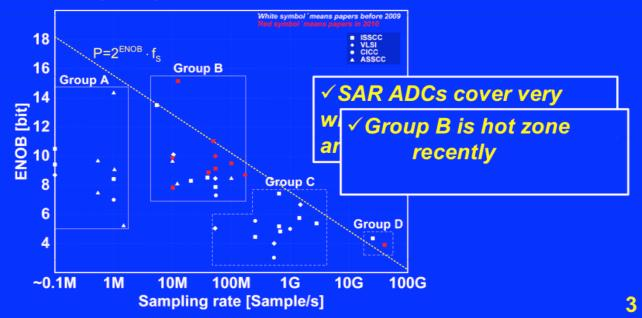
Source : A 550uW 10b 40MS/s SAR ADC with Multistep Addition-only Digital Error Correction, *Sang-Hyun Cho et al.* CICC 2010 *(FOM = 42fJ/conversion)* designed in 0.13um CMOS
