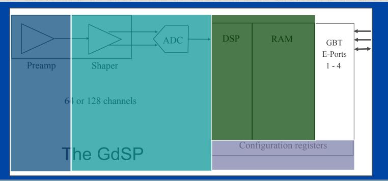
Preamp > Reduce current via bias control, important to maintain a low impedance on the electrode.
