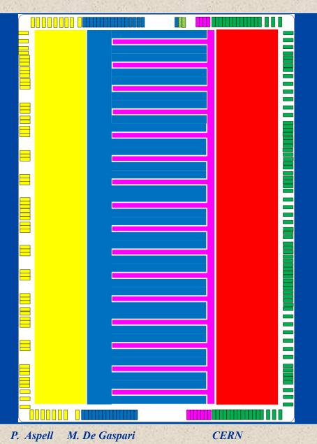
Power domains: PASA analog ADC analog ADC digital Digital core Digital Pads
