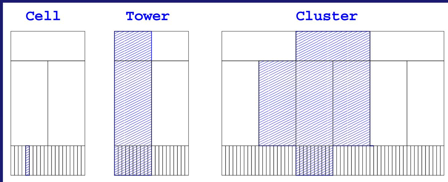
▶ A tower is a group of cells (or even a group of fractions of cells) in a fixed  $\Delta\eta \times \Delta\phi$  grid over some or all samplings
