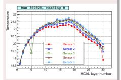
Problematic sensors flagged as 'bad' and removed, use median of 'good' sensors instead
