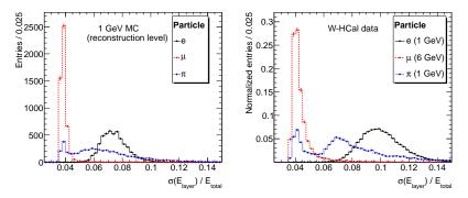
$\Rightarrow$  Can have a handle for particle selection based on Cherenkov triggers and on selected variables ('shower depth', 'uniformity of energy loss') also at low energies
