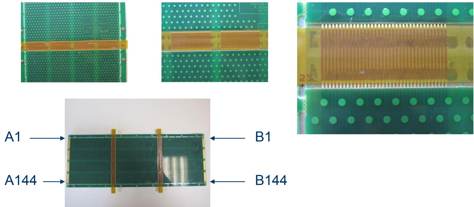
A first test taken between points A1 to A144 and B1 to B144 shows that continuity of 2x4 connectors 36 channels is established
