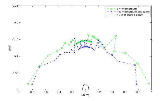
Dynamic aperture is much larger then the size of stored beam and is enough also for an off-axis injection system and top-off operation.
