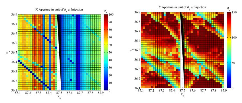
Dynamic aperture in a two-dimensional tune scan for the baseline design of PEP-X.
