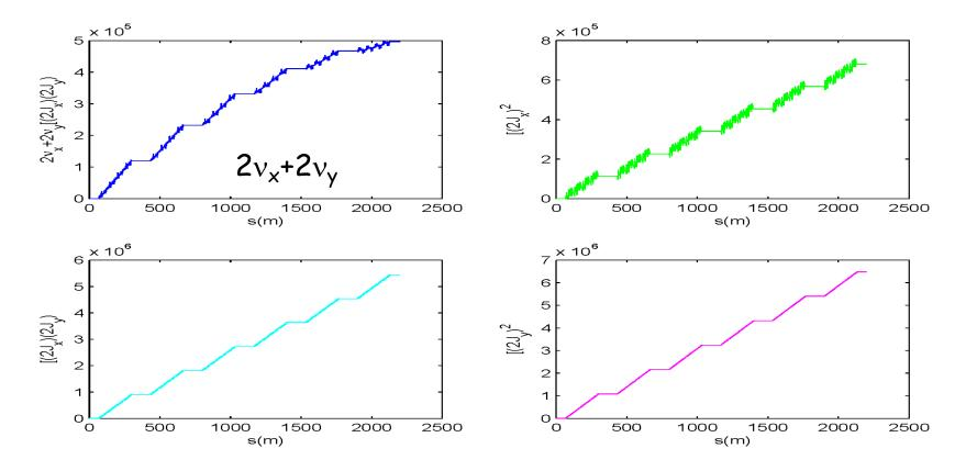
Interferences among sextupole magnets, calculated using LEGO. The results show that eight 135°/45° cells generate a systematic 4<sup>th</sup> order resonance, namely  $2_{Vx}+2_{Vy}=258$ .
