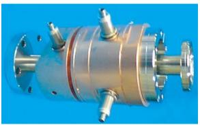
Cavity BPMs, for use with Q magnets with 100nm resolution (PAL, SLAC, KEK)
