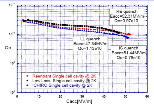
Figure 3: The results of high gradient measurements.
