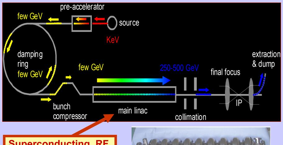
Superconducting RF Main Linac
