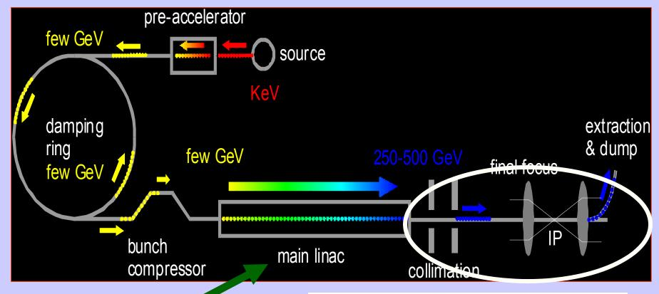
Superconducting RF Main Linac
