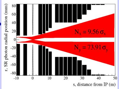
Example of SR rays from beam halo in IR apertures
