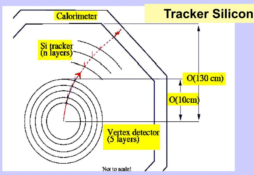
5 layers of pixel detectors and 5 layers of Si-strip
