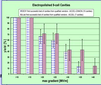
Note: These are results from the vertical CW test at DESY and JLab
