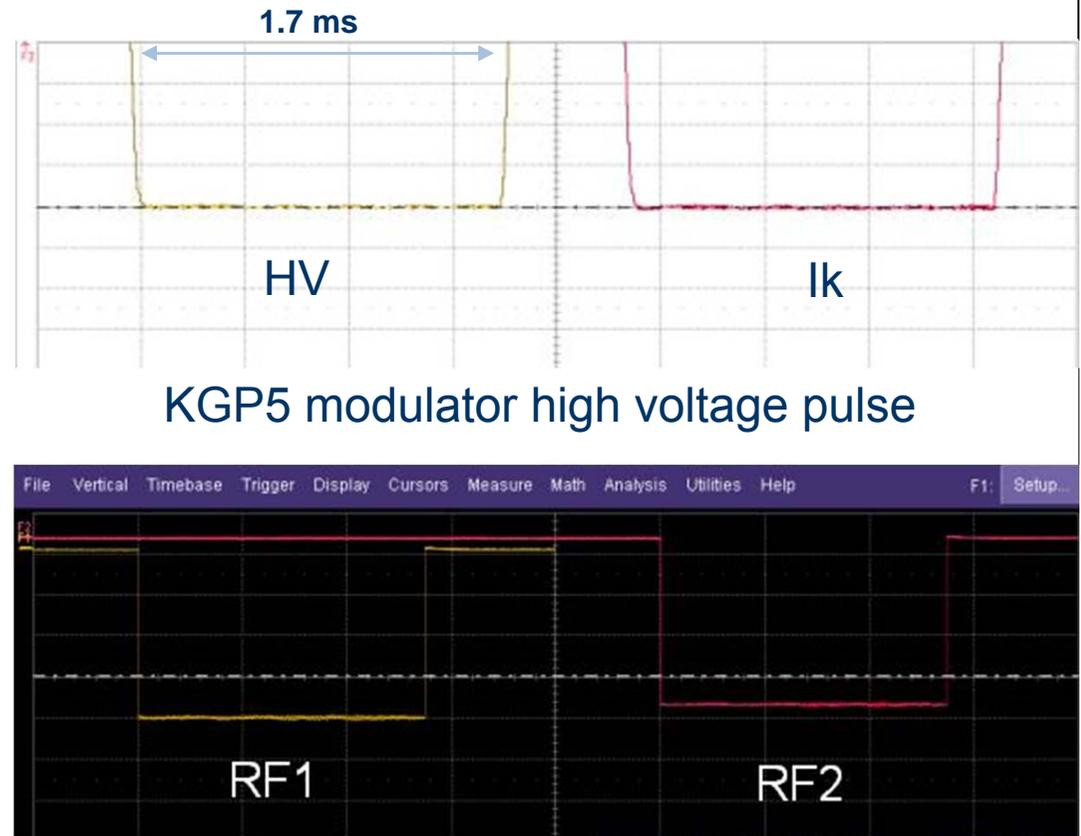
**10 MWp Output power at 116 kV in long pulse (1.5 ms RF)**
