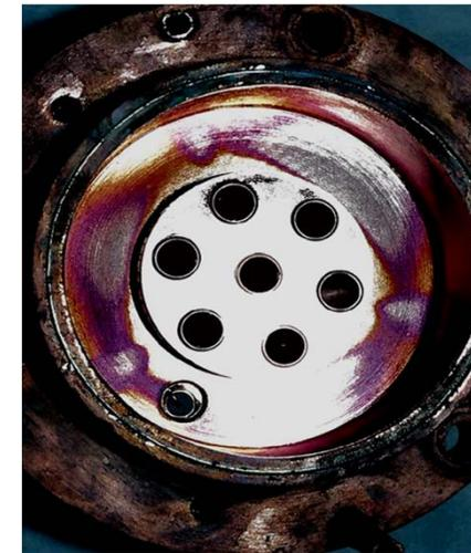
Heated cavity after HOM oscillation
